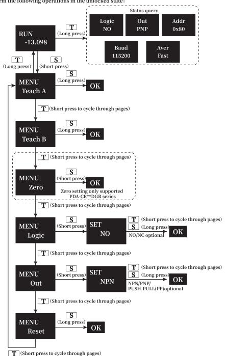
3.Setting waiting interface: When long press S key to set, you will be prompted with three solid dots to indicate the setting progress (Take Teach A as an example):
