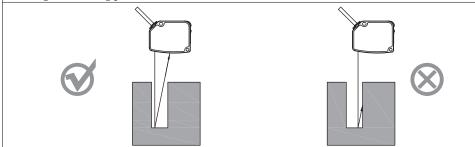
Measurement for wall surface mounting(Install in the direction shown in the figure below to reduce the multiple reflected light from the wall surface, since the reflected light will enter the receiving surface. In case of wall surface high reflection rate, it is better to change to matter black)
