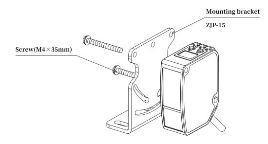
\*For mounting, please keep tightening torque < 0.5N·m
