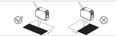
Step surface or segment gap measurement(Install in the direction shown in the figure below to reduce impact by step edges in measurement)
