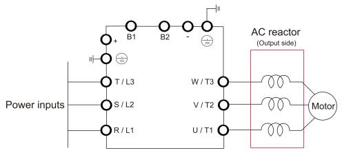
Figure 6-6 Connecting an AC Output Reactor
