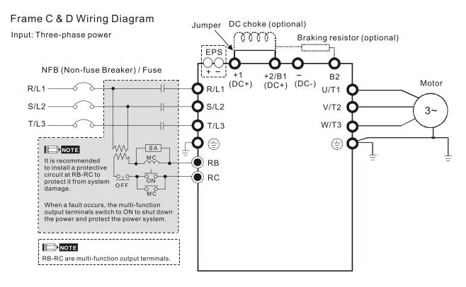
Figure 6-5 Installing a DC Reactor
