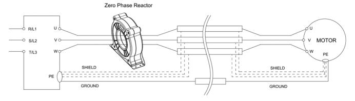
Figure 6-32 Single turn wiring diagram for shielding wire with a zero phase reactor
