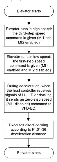
The steps to execute direct docking terminal function using deactivating multi-step speed command 1 and 2 (MI1 and MI2) are as follows:
