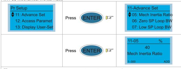
You can calculate the load inertia according to the settings of motor parameters, Pr.11-01 to Pr.11-04 and Pr.11-14 Motor Current at Acceleration and Pr.11-15 Carriage Acceleration. You can use this parameter to adjust the mechanical inertia ratio.
