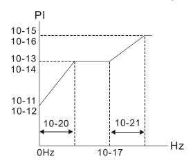
When using multi-function input terminals to switch ASR1/ASR2, the following diagram shows the operation.
