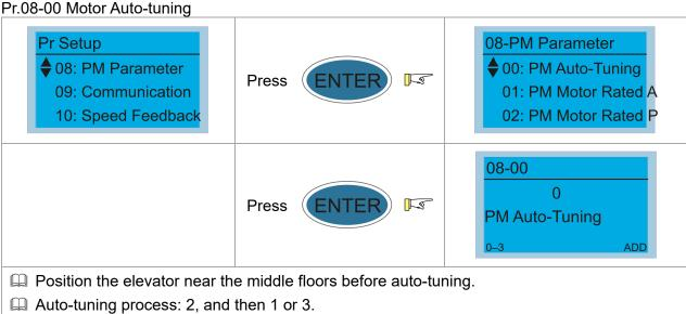
Set Pr.08-00 to 1 to 3, and then press the RUN key on the digital keypad KPC-CC01 (Pr.00-15=2) to start auto-tuning. Or when the drive is in manual mode (inspection), run the upward operation or downward operation (Pr.00-15=1) to start auto-tuning immediately. In the
