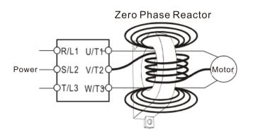
Figure 6-33 Multi-turn zero phase reactor
