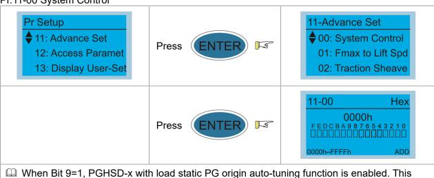
function is valid only when the mechanical brake is in engaged status.
