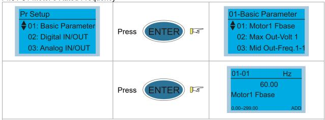
Set this parameter according to the rated frequency on the motor nameplate. If the motor is 60 Hz, set this parameter to 60. If the motor is 50 Hz, set it to 50.
