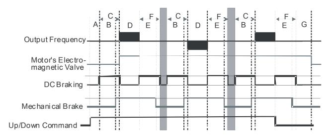
A Pr.02-31: Magnetic Contactor Contracting Delay Time between Drive and Motor
