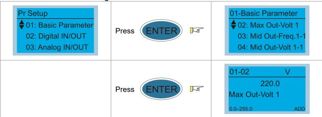
Set this parameter according to the rated voltage on the motor nameplate. If the motor is 220 V, set this parameter to 220.0. If the motor is 200 V, set this parameter to 200.0.
