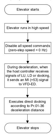
The steps to execute direct docking terminal function using multi-function input terminal (MI=53) are as follows:
