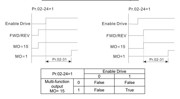
After both Enable Drive function signal and MO15 output, the drive starts to count Pr.02-31.
