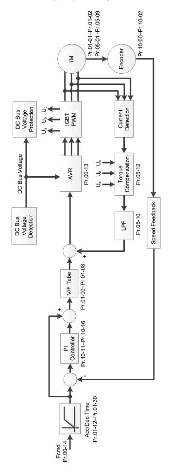
When Pr.00-09=2, Sensorless Vector Control (SVC) control diagram is as follows:
