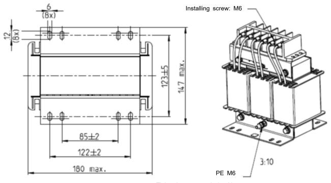
Tightening torque: 3±1.5 Nm
