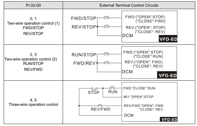
Multi-function Input Command 1 (MI1) (It is the Stop terminal for three-wire operation)
