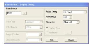
Click [...]. In the **Refer Device** dialog box, choose the VFD communication port that you need. If you want to read the output frequency (H), set the **Absolute Addr.** to 2202. For other values, refer to Appendix B-4 ACMD Modbus Comm Address List in this user manual.
