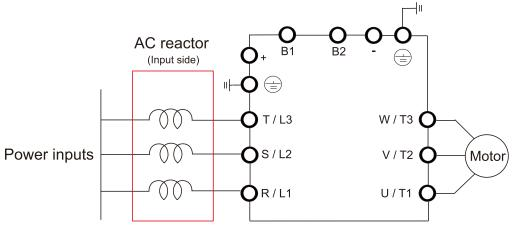
Figure 6-4 Connecting an AC Input Reactor
